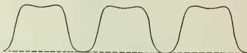
FIG. 92.—DIAGRAM OF A POSSIBLE WAVE FORM OF MAGNETO-ELECTRIC GENERATOR E. M. F. (WHEN A COMMUTATOR IS EMPLOYED).
